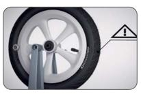
Align the front tire between the front fork ensuring that the tire rotation direction matches the rear tire and directional arrow on the tire. The recommended / maximum tire inflation pressure is **2,5 bar** (36.25 PSI). DO NOT OVER-INFLATE!
