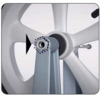
Insert the self-locking nut (Part E) into the hexagonal hole on the left side of the fork and insert and tighten the wheel bolt (Part D) from the right side using the hexagon ("Allen") wrench (Part F).
