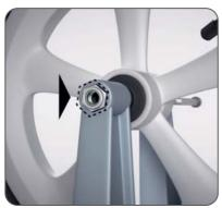
Insert the self-locking nut (Part F) into the hexagonal hole on the left side of the fork and insert and tighten the wheel bolt (Part E) from the right side using the hexagon ("Allen") wrench (Part G).
